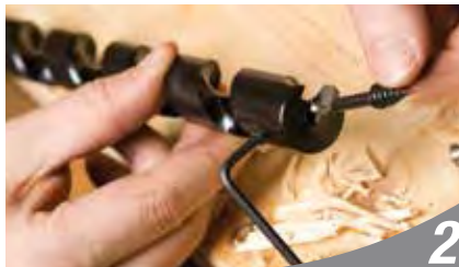
Insert Feed Screw...
