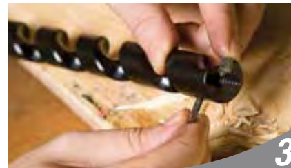
Tighten Set Screw.
