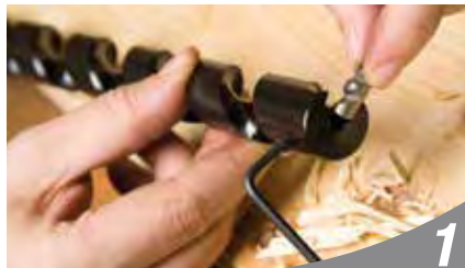
Insert Cutting Edge...
