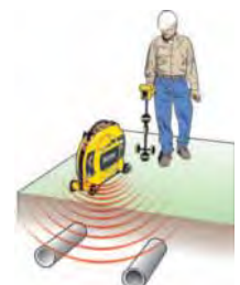
Induce a signal to locate utilities.
