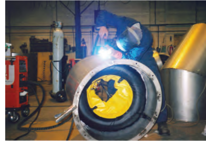
Rapid Purge used to weld a stainless steel elbow.
